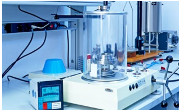
Piston manometer in the calibration laboratory of the Walcher Meßtechnik GmbH
