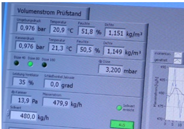
The calibration test stand collects and documents volume flow and mass flow measurements in highest precision.
