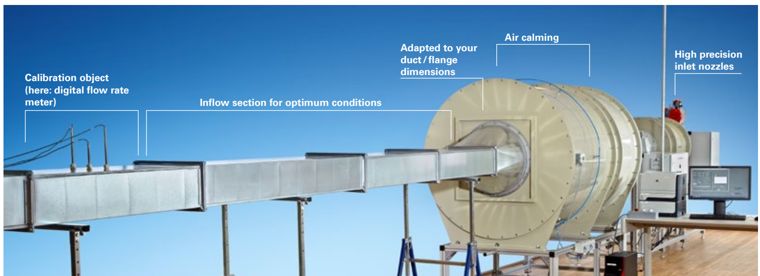
High precision inlet nozzles for accurate measurement results
